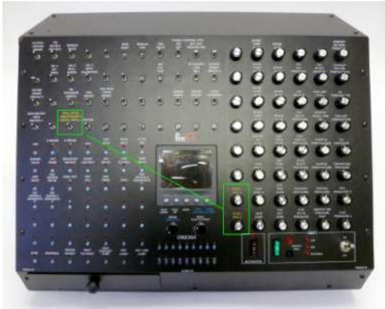
**Dual Pedal Position Sensor:** For ECM's with dual PPS inputs, there are 2 pots and 1 switch used to control the load box outputs. When the switch is in the UP position, the PPS1 and PPS2 pots are used to control the corresponding ECM inputs. When the switch is in the DOWN position, the PPS1 pot is used to control both PPS1 and PPS2 outputs. In this case, PPS2 voltage is automatically adjusted to  $\frac{1}{2}$  PPS1 to prevent PPS1/PPS2 mismatch faults.
