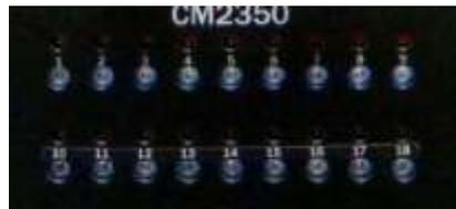
**Injector Indicators:** There are 18 simulated injector loads inside the load box. The LED's shown above indicate when each injector fires. The associated testpoint provided a voltage representation of the injector current. This output is scaled as shown below:
