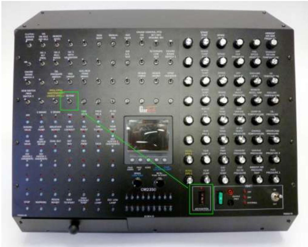
**Keyswitch:** The keyswitch fuse (7.5A) is located on the front panel along with an LED indicator. The switch is always wired in the harness to the location shown above.
