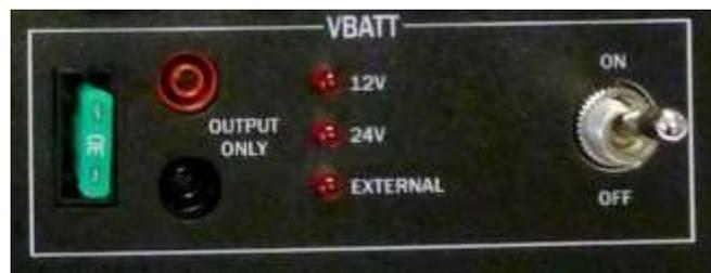
**VBATT:** VBATT is fused at the front panel (30A). The banana jacks here are connected to VBATT and also go thru the 30A fuse. The LEDs indicate if the 12V or 24V internal supply is selected. If an external VBATT supply is connected to the load box, the EXTERNAL LED is active. The ON/OFF switch is used to enable/disable VBATT connection to the ECM.
