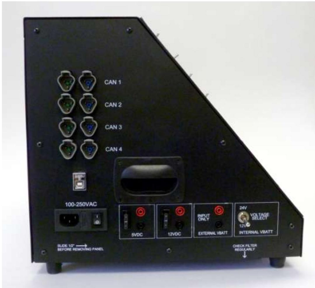
**AC Power:** The ULB accepts 100-250VAC input. The 6.0A / 250V AC power fuse is located between the power switch and the power cord attachment behind the small plastic door.
