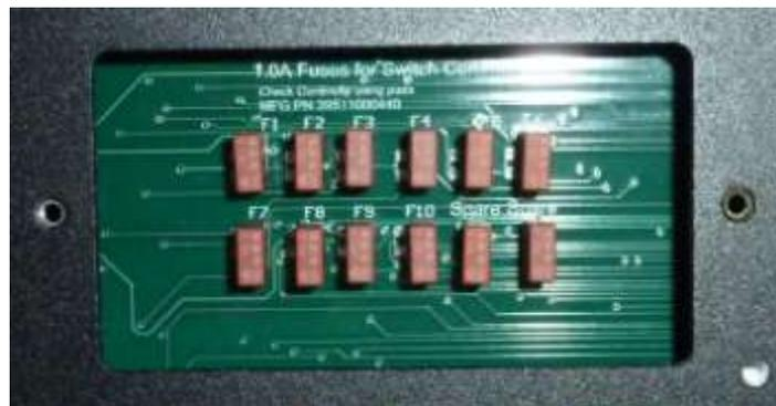
**Switch Fuses:** These fuses are found behind the “Switch Fuse Panel” cover on the back side of the load box. Note that 2 spare fuses are included.
