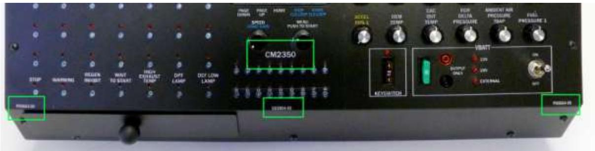
**Overlay Identification:** Overlays are available for each ECM. Customized overlays suited to your particular application are also available. The ECM/application ID is located above the injector testpoints. The overlays are created by placing 2 vinyl pieces onto an aluminum backing. Each vinyl half has a part number shown above in the bottom left and bottom right corners (Pxxxxx-xx). The overall PN (Gxxxxx-xx) for the complete assembled overlay is in the middle, below the injector testpoints.
