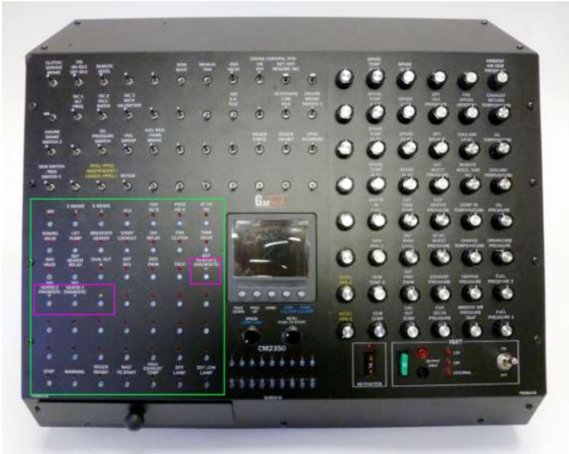
**Loads:** Each internal load has an LED on/off indicator and high-side voltage testpoint on the front panel. There are (4) bidirectional indicators outlined above. These LED's turn RED or GREEN depending on the direction of current flow through the load.
