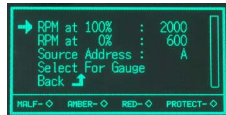
Figure 23. J1939 Throttle Setup
